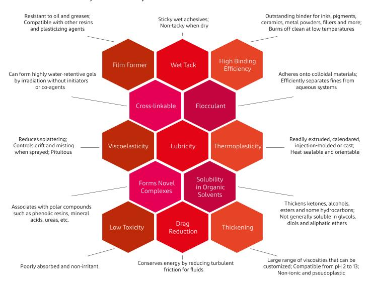
Films of POLYOX™ WSR are flexible, tough and resistant to most oils and greases With their very high molecular weight, POLYOX™ WSR polymers are viscoelastic, so their aqueous solutions can reduce spattering and misting.
